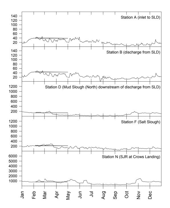
**Figure 2.** Comparison of monthly selenium load discharge from the terminus of the San Luis Drain (Station B) with the monthly load values in the Interim Use Permit for calendar year 2007.
