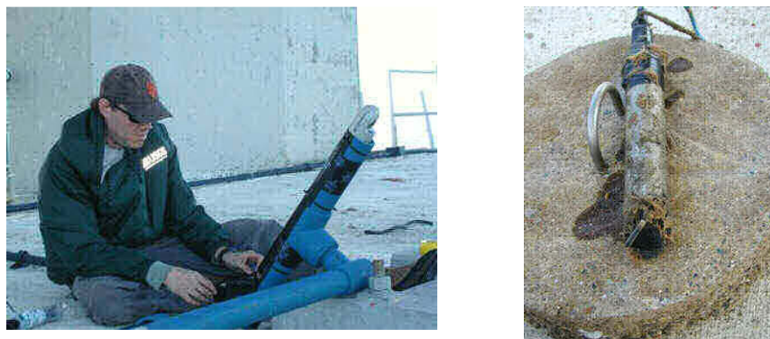
Figure 4. Left: An acoustic Doppler current profiler (ADCP) measured water speed and direction. Right: An optical turbidity probe measured turbidity, a surrogate for direct measurements of suspended sediment concentrations. Greg is working on getting better pics.
