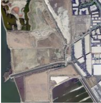
Figure 1. Aerial photo of the Zone 4 Line A channel and outfall at Hayward Landing. In this case sediment has built up in the channel a lateral bar deposit from the Bay to a distance of 1 km upstream (about 2/3 of the width of this photo image).
