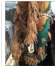
RMP water quality sensor playing host to animals called hydrobots. Photo by Emily Novick, SFEI.
