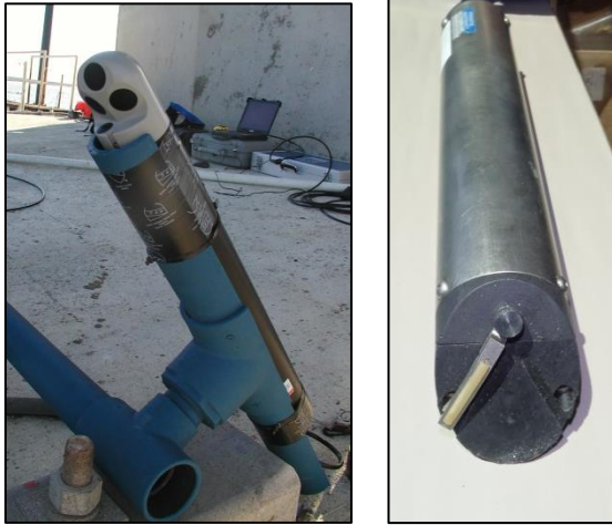
Figure 4. Left: An acoustic Doppler current profiler (ADCP) measured water speed and direction. Right: An optical turbidity probe measured turbidity, a surrogate for direct measurements of suspended-sediment concentrations. Do we need better pictures?
