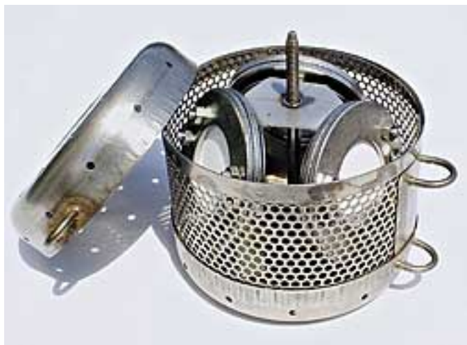
Figure 1. Deployment holder featuring one POCIS holder containing three POCIS. Dimensions 15 cm high x 16 cm wide. Environmental Sampling Technologies, est-lab.com
