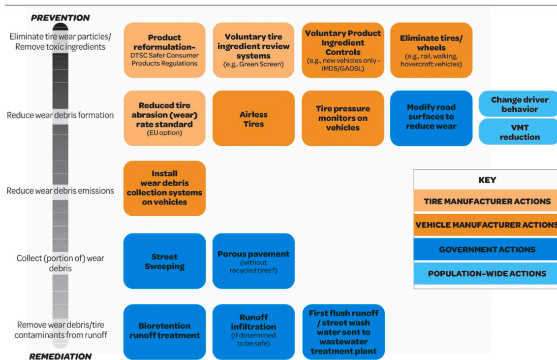
Fig. 4. Management options for tire wear particle pollution, framed on a scale from preventative (reducing use and release) to remedial (collection and removal) measures. Options are color-coded by who would be responsible for implementation, with tire manufacturers in light orange, vehicle manufacturers in dark orange, government in dark blue, and community-wide in light blue. Reprinted from Moran et al. (2021).
