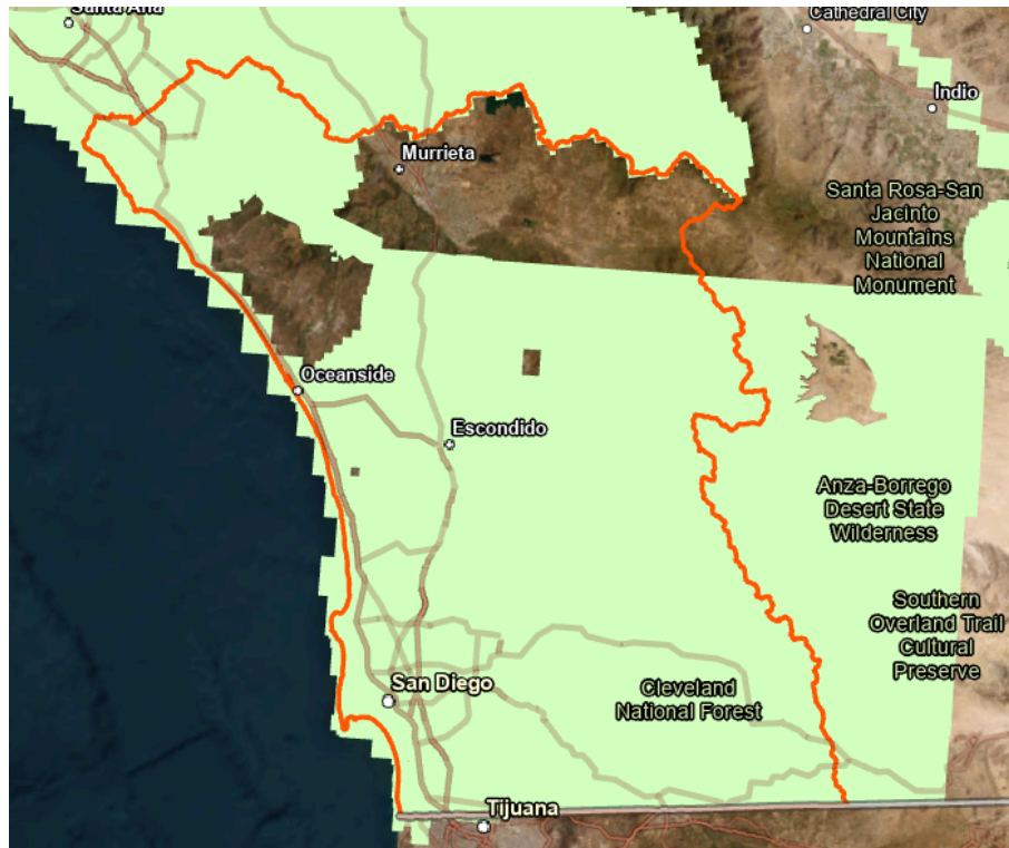
Figure 7. High resolution lidar coverage is shown in light green, with the SDARI study area boundary shown in orange. Areas not covered by the light green and showing the underlying imagery are where supplementary lower resolution lidar was used. Approximately 450,500 acres, or 18%, of the SDARI study area didn't have high resolution lidar available at the time of mapping.
