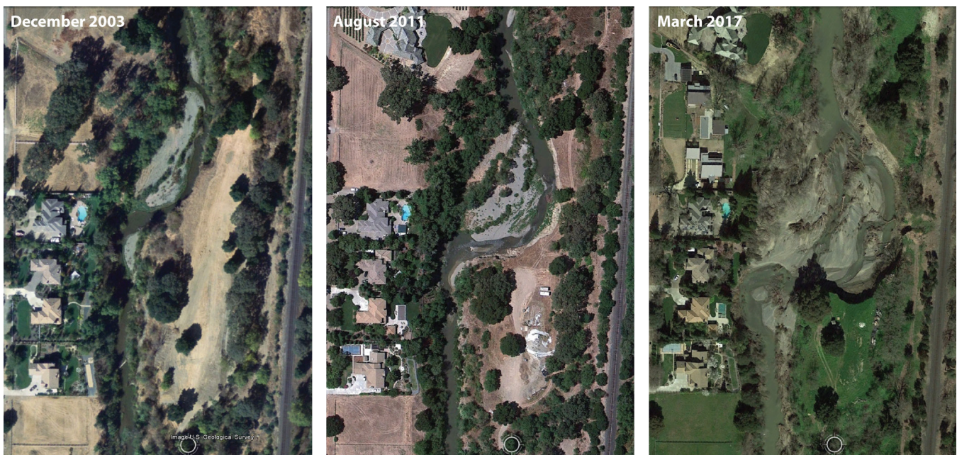
Figure 12. Time series of aerial photographs illustrating the migration of the channel meander at the downstream S-curve.
